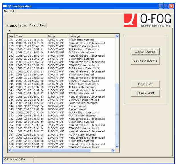
The CPU board has a log buffer that saves the latest 256 entries. Data in this buffer is not erased in case of a power failure. A log entry showing the time of the power failure is created and stored in the buffer.
