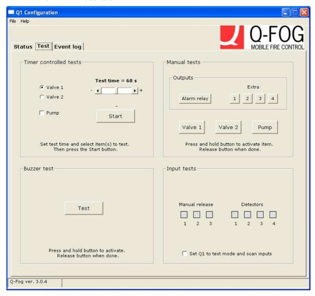
This window is used for testing the functionality of control boards and complete sprinkler units.
