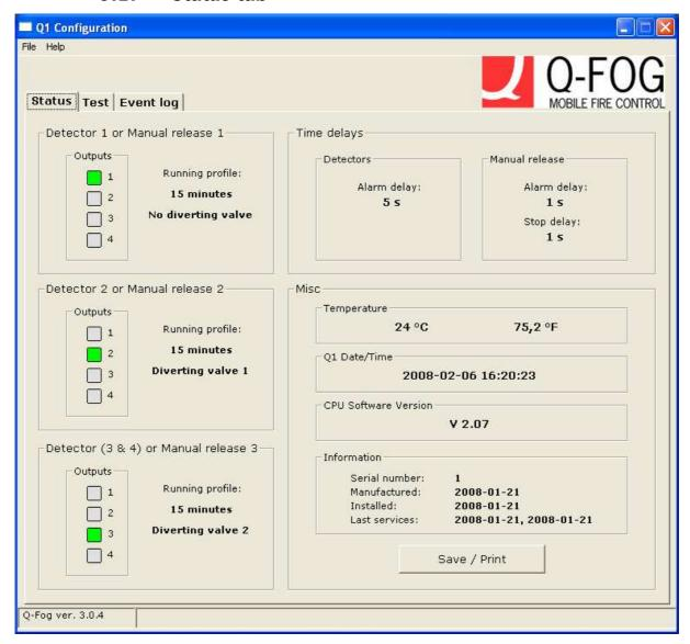
This window tells the status of all the settings of the actual system connected to the PC.
